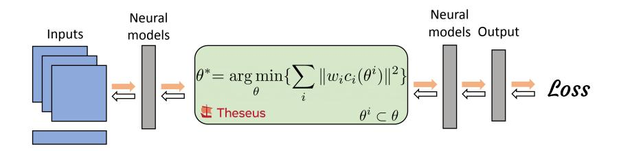
Theseus is a library for building custom nonlinear optimization layers in PyTorch to support constructing end-to-end differentiable architectures
