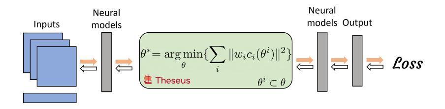
Theseus is an efficient application-agnostic library for building custom nonlinear optimization layers in PyTorch to support constructing various problems in robotics and vision as end-to-end differentiable architectures
