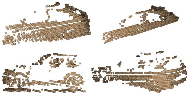
“car” objects cropped from LiDAR point cloud
