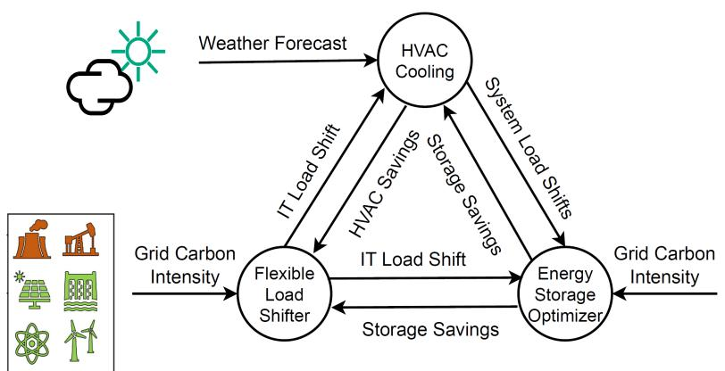
Internal and External Dependencies for the Cooling, Load Shifting and Battery agents
