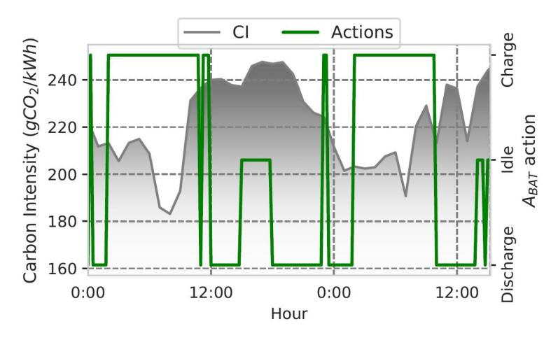
Sample time slice demonstrating the incremental carbon footprint savings using C2FR. We observe that the battery considers both the carbon intensity and the spikes in load to discharge and reduce carbon footprint.
