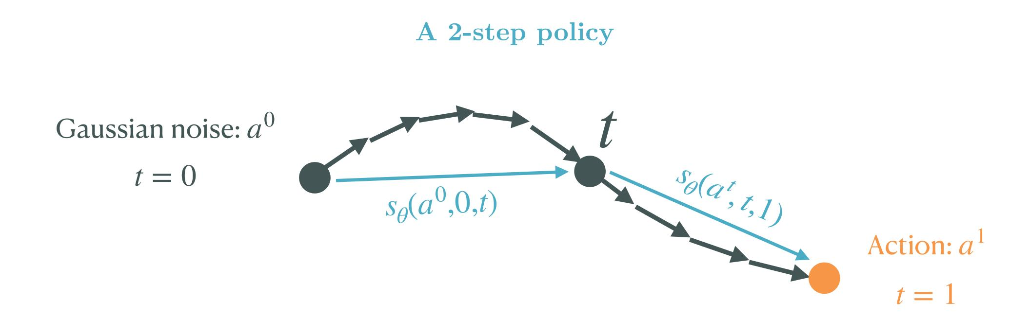
$s_{\theta}$ : a differentiable function modeling a jump for some time interval t
