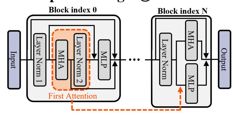
**FAL** redirects the MLP input from the current MHA to the first attention, replacing the redundant per-block MHA→MLP dependency
