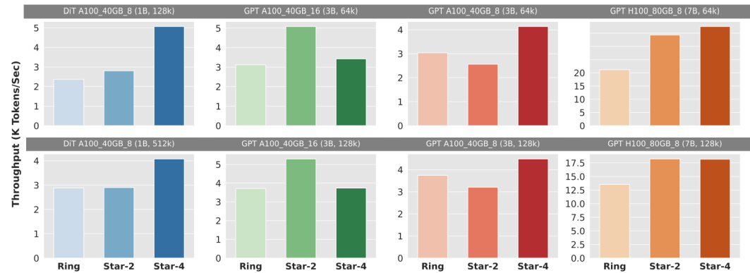
Figure 7: Throughput evaluation of Ring Attention and StarTrail on 32 GPUs from three different clusters. We place the performance of StarTrail with both C=2 and C=4 in the figure. The configurations are marked in the titles of the sub-figures. For instance, A100_40GB_8(1B, 512K) represents that the experiment is on machines with 8 Nvidia A100 40GB GPUs in each node, the model used has one billion parameters, and the sequence length is 512k.
