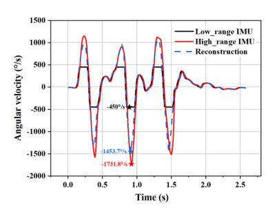
Extends measurable range from  $\pm 450^{\circ}$ /s to  $\pm 1500^{\circ}$ /s
