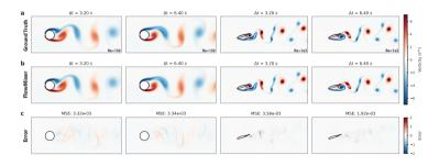
Vorticity  $\omega$  for Cylinder (Re=150) & airfoil (Re=1000): prediction horizon 6.4 s **16× speedup** vs spectral solvers | Relative error:  $\sim$ 4% | Purely data-driven
