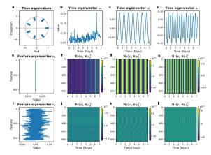
Eigenmodes of Traffic dataset showing base trends and daily/weekly cycles. Coupling reveals propagation patterns.
