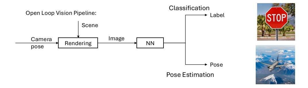
• Safety/Verification Question: Given continuous variations in camera poses and scene configurations, determine the regions where a trained image-based neural network reliably outputs correct predictions and where it does not.
