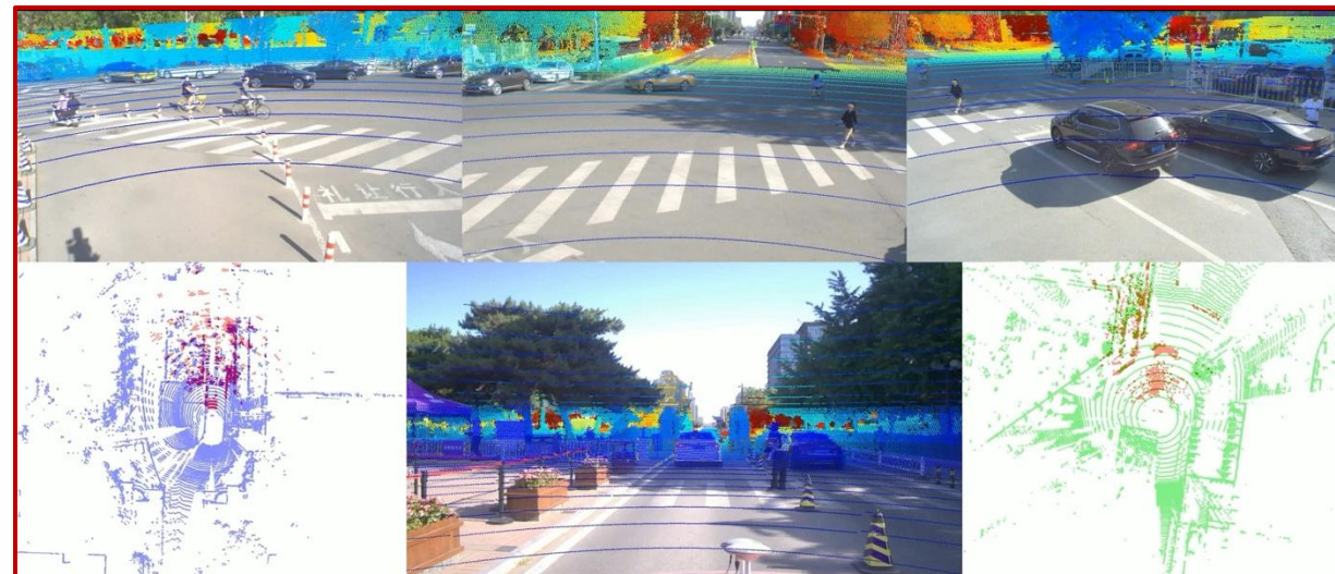
Visualization of single-agent sensor calibration results
