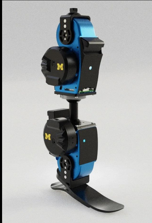
MyoOSL Finite-state machine, 2 actuators 4 Degree of Freedom (DoF)
