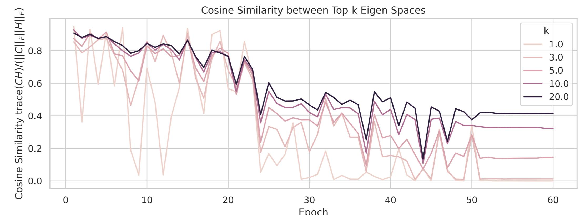
There exists a non-trivial level of correlation between the covariance matrix  $C$  of the gradient noise and Hessian  $H$  (though decreasing).
